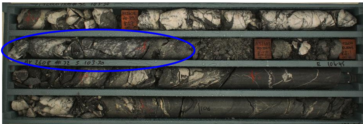
Figure 10: AY2608 Tray #32 with an example of quartz breccia with stibnite infill.
