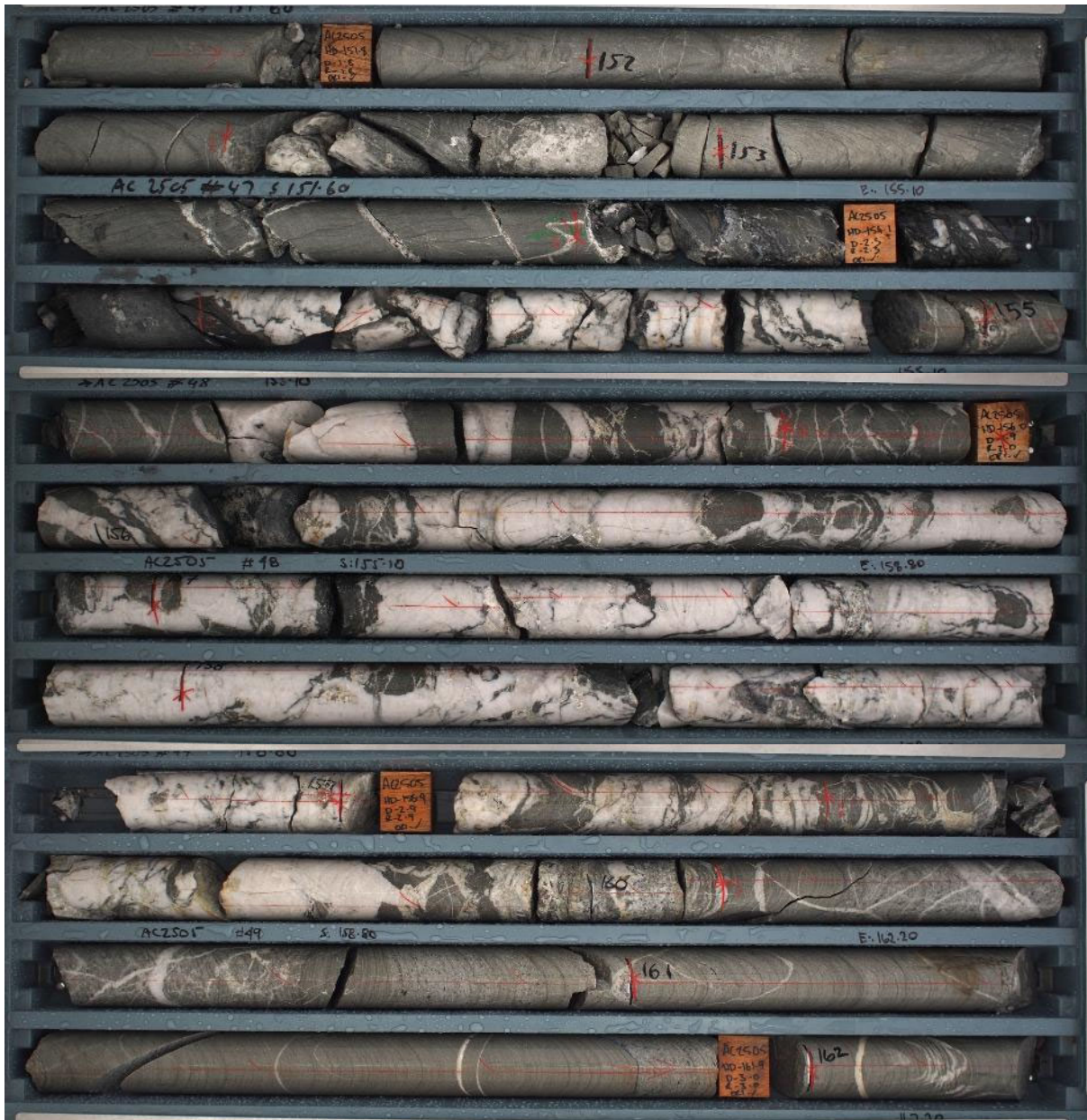
Figure 3: AC2505 Tray #47, #48, #49 (151.6m to 162.2m) showing stylonitic quartz
