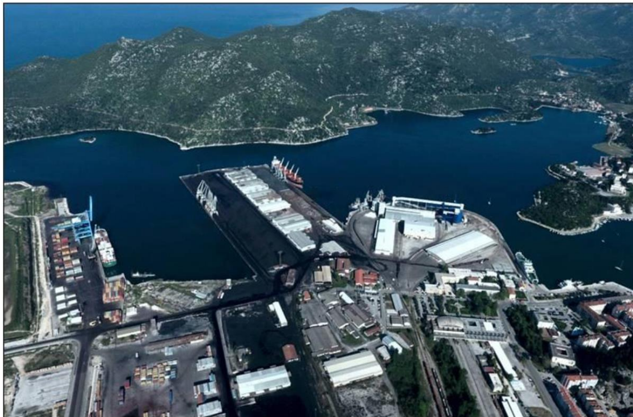
Figure 15: Aerial view of the Ploce Port. The container terminal is on the left-hand side. The other 4 quays are bulk terminals. (Photo: Wilhelmsen Ship Service 2021)
