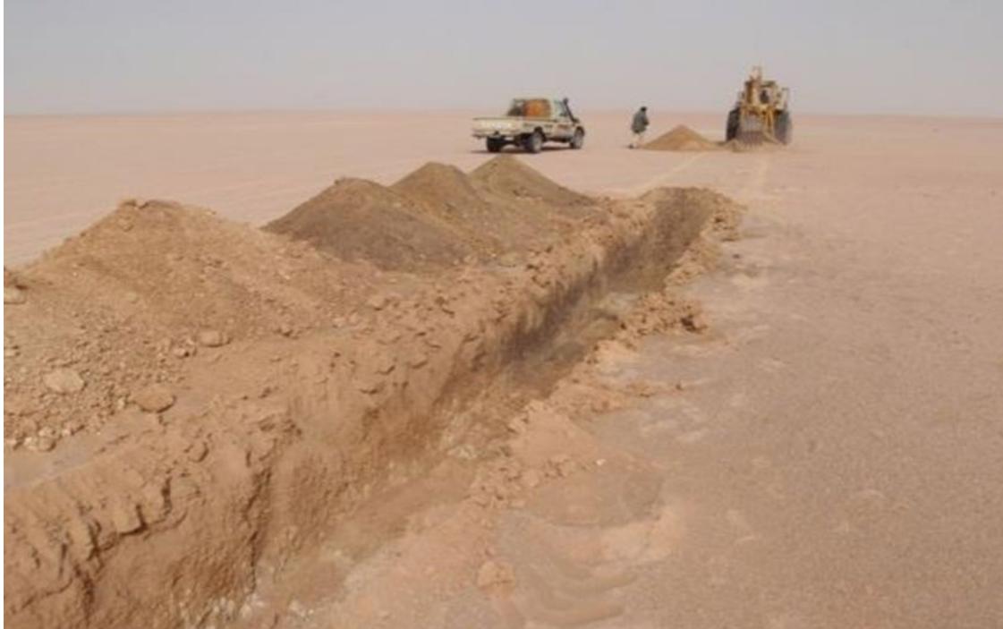
Figure 7: Typical trench showing soft sandy overburden over gravelly, free-digging calcrete ore
