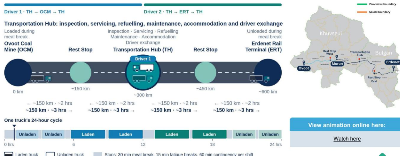
Figure 4: Planned 24-hour trucking circuit from the Ovoot Coal Mine to the Erdenet Rail Terminal. Watch the animation on YouTube
