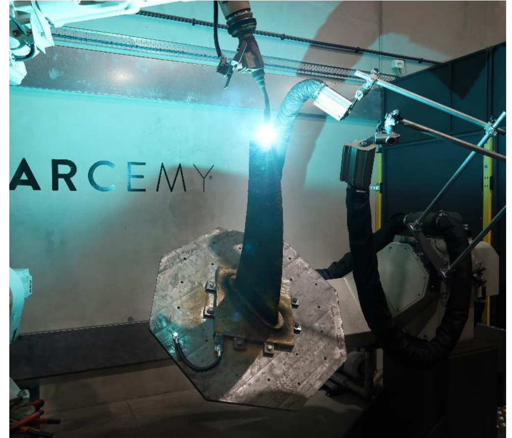
WAM® Nickel Aluminium Bronze Propeller Blade.
