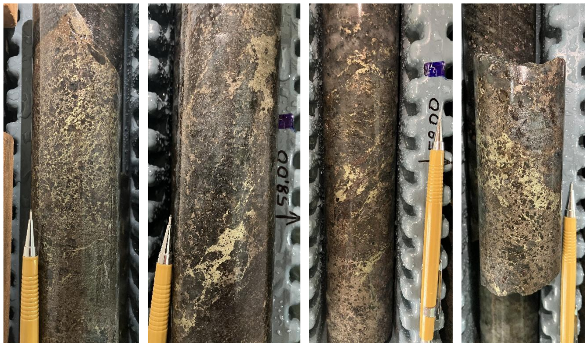
Figure 4: Mineralised intervals at Touro Prospect. From left to right: PDT-117 from 56.75m downhole, PDT-117 from 57m downhole, PDT-117 from 58m downhole and PDT-117 from 64.2m downhole. Dark brown mineral is sphalerite (zinc sulphide), golden colour is chalcopyrite (copper sulphide), pale yellow is pyrite (iron sulphide) and bronze colour is pyrrhotite (iron sulphide).
