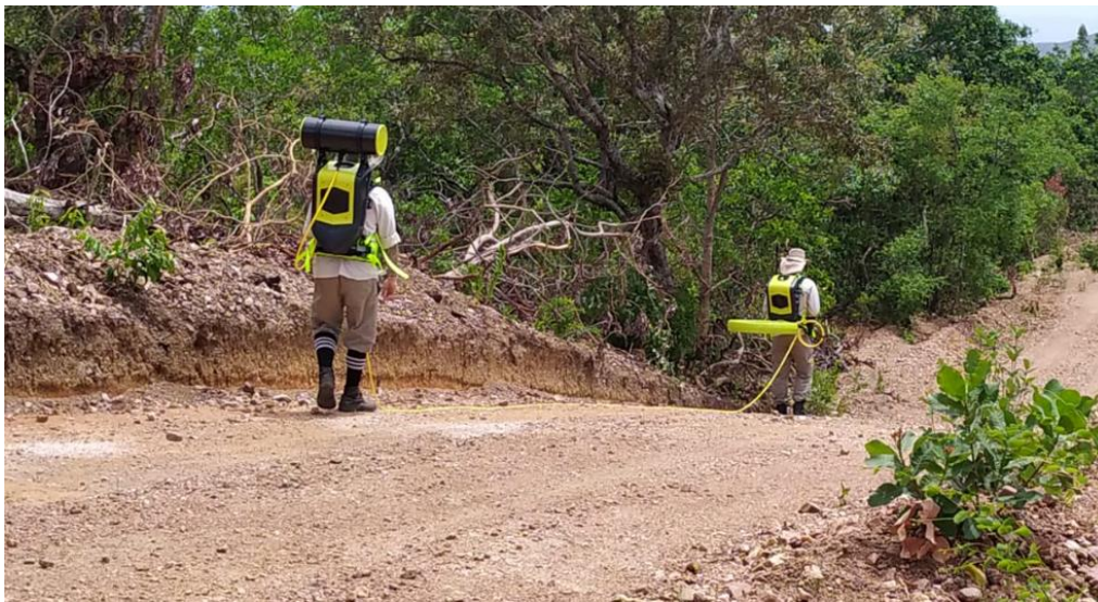
Figure 3: Loupe portable electromagnetic survey underway at Bluebush.
