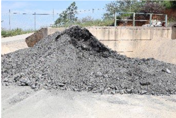
Figure 1: Crushed mineralised material stockpile (approximately 200 tonnes) and stockpile sampling for ore control and laboratory assay
