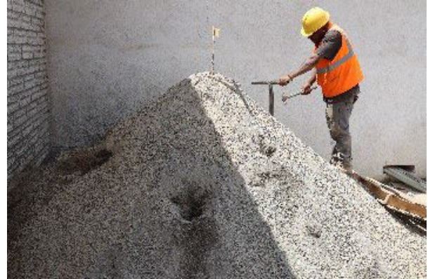
Figure 1: Crushed mineralised material stockpile (approximately 200 tonnes) and stockpile sampling for ore control and laboratory assay
