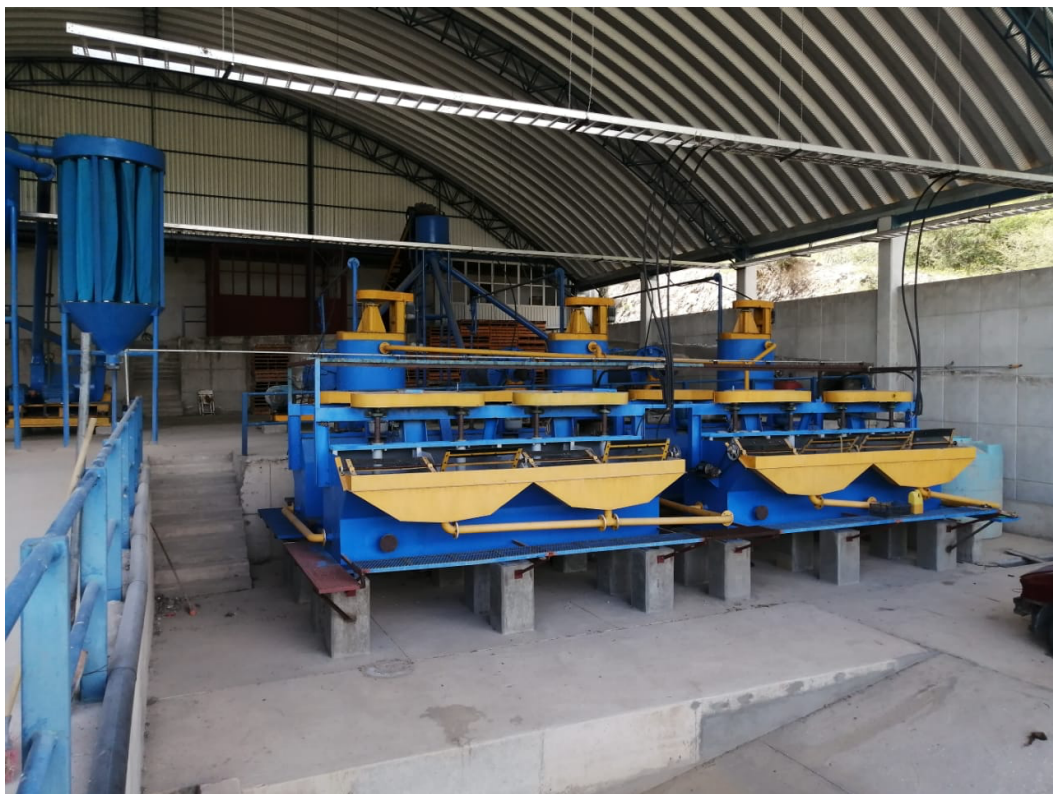
Figure 2: Flotation cell banks at the Tecamatlán Processing Plant.
