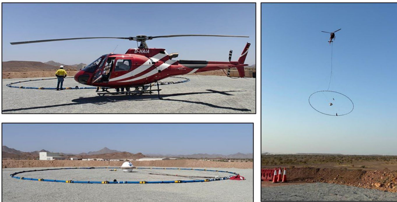
Figure 5 – HeliTEM Airborne Electromagnetic Survey in Action
