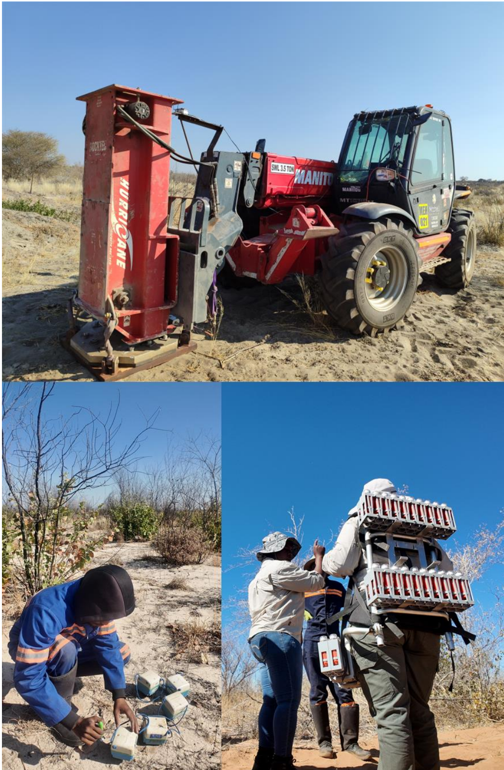
Figure 1. (Top) 1.5t accelerated weight drop source; (lower left) Smart Solo passive seismic node layout; (lower right) Stryde™ active seismic node deployment.
