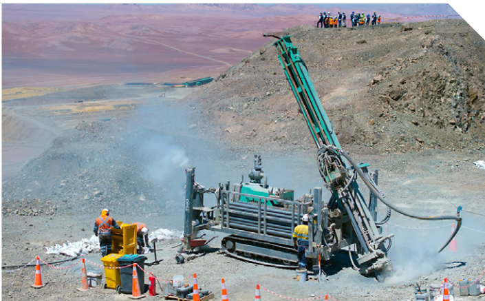
Figure 13 | Reverse-circulation drilling at the open-pit oxide resource, Sierra Atacama
