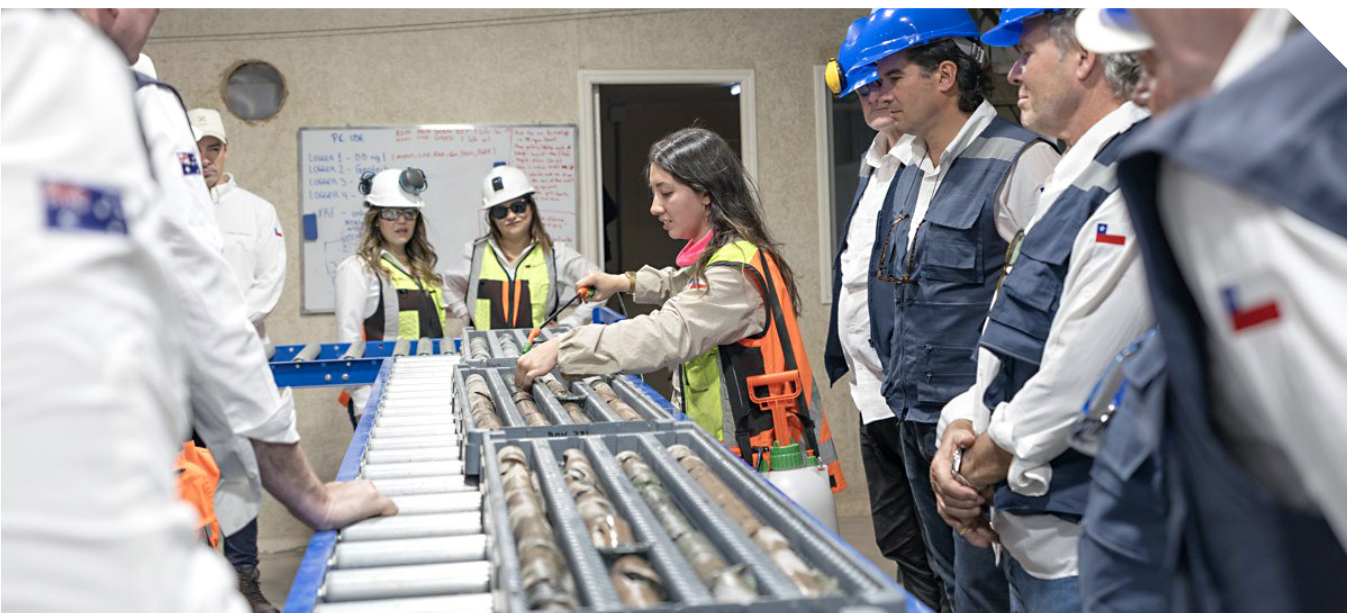
Figure 15 | The geology team logging drill core at the rebuilt core sheds.
