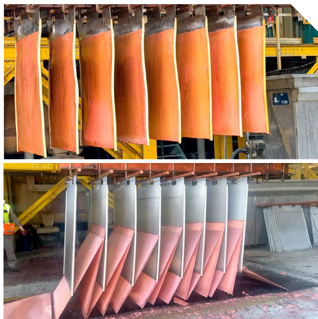
Figure 8 | Cathode plates before (top) and after (bottom) replacement with new stainless-steel-body plates – straighter, more uniform and higher purity.
