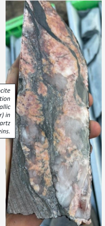
Hydrothermal breccia with chrysocolla (and fine-grained chalcocite) mineralisation
