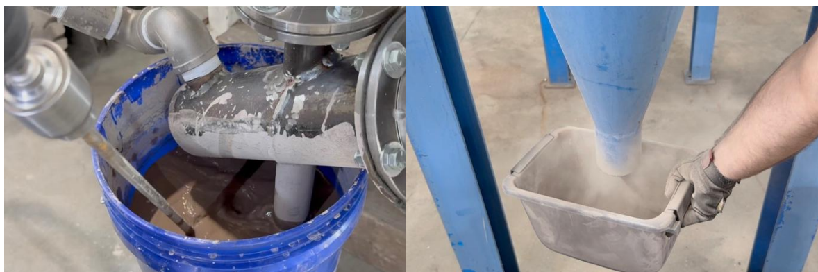
Drying of slurry directly from 40% moisture to <0.5% moisture.
