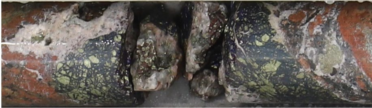
Figure 3. Sample 20TR1665 from hole DEVO0018 returned an inductive conductivity reading. Late matrix chlorite-bornite and chalcopyrite breccia in quartz-carbonate vein breccia from 687.66m – 687.82m assaying 5.37% Cu, 0.03g/t Au (see ASX release 2 August 2023).
