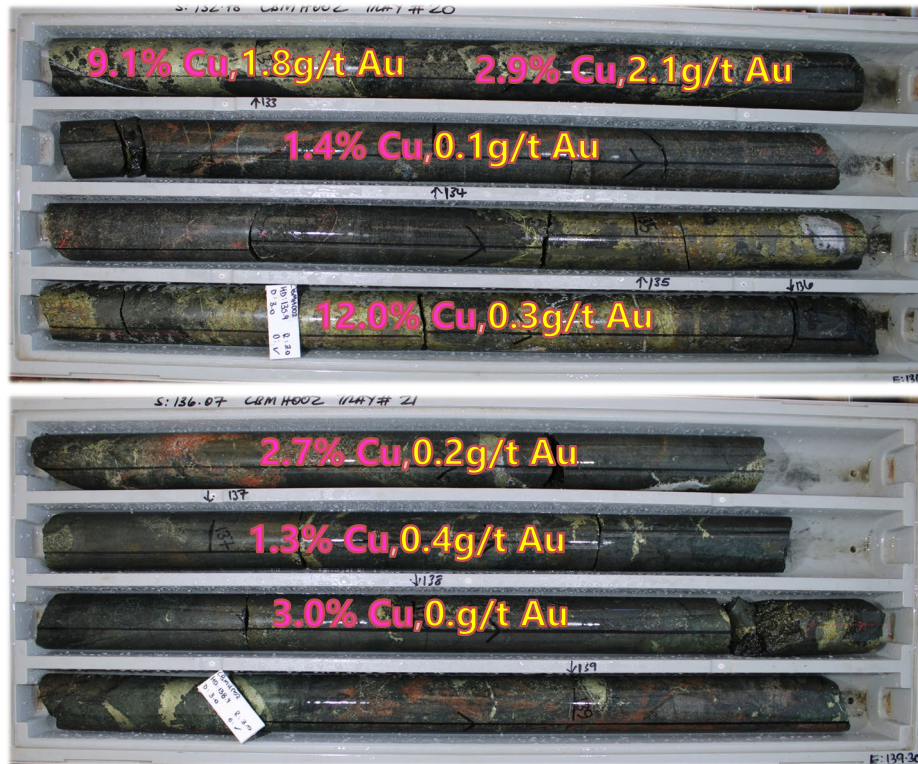
Figure 3. CBMH002 core showing high grade copper gold mineralisation from 128.6m to 139.1m which averaged 4.1% Cu, 0.8g/t Au.
