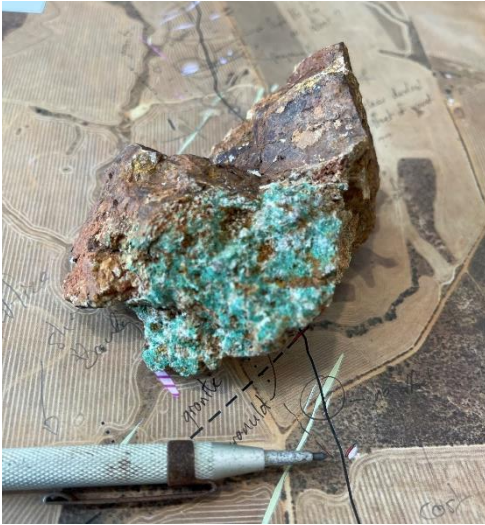
Figure 3: Sample from the southern end of Yungaro: malachite with vuggy carbonate on oxidised dolerite taken from sub-crop proximal to historical costeans.
