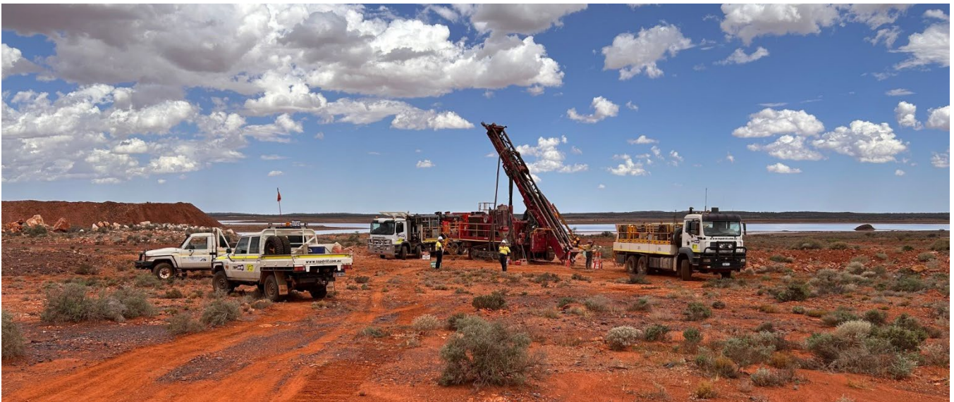
Figure 1. Topdrill track mounted RC23 drilling at the Island Gold Project February 2025.
