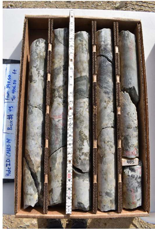
CM24-14 drill hole core. Estimate of sulphide content is 20%
