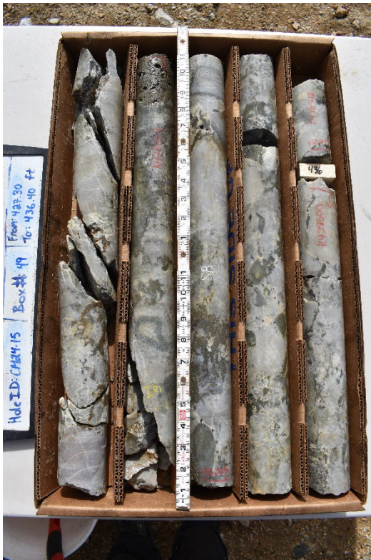
CM24-15 drill hole core. Estimate of sulphide content is 20%
