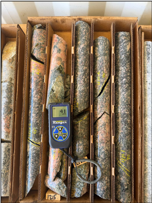
Figure 3: CE26-05 - 1215-1217 feet – interstitial calcite
