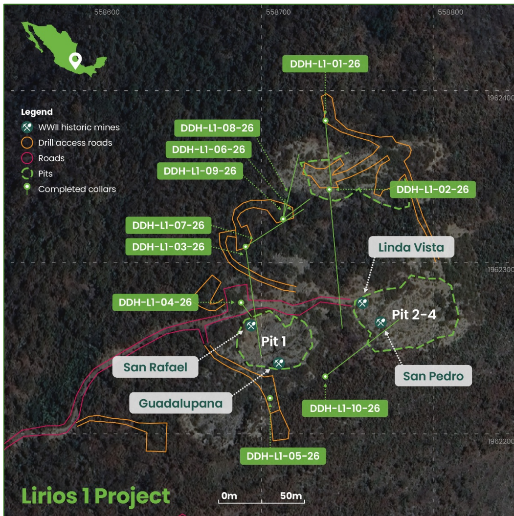
Figure 5: Lirios 1 Historical Adits and pits with Phase 1 drill collar location
