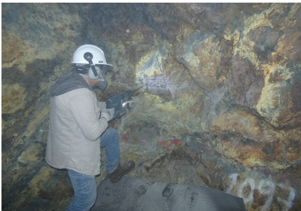
Photo 5. Channel Sample Being Cut Underground
