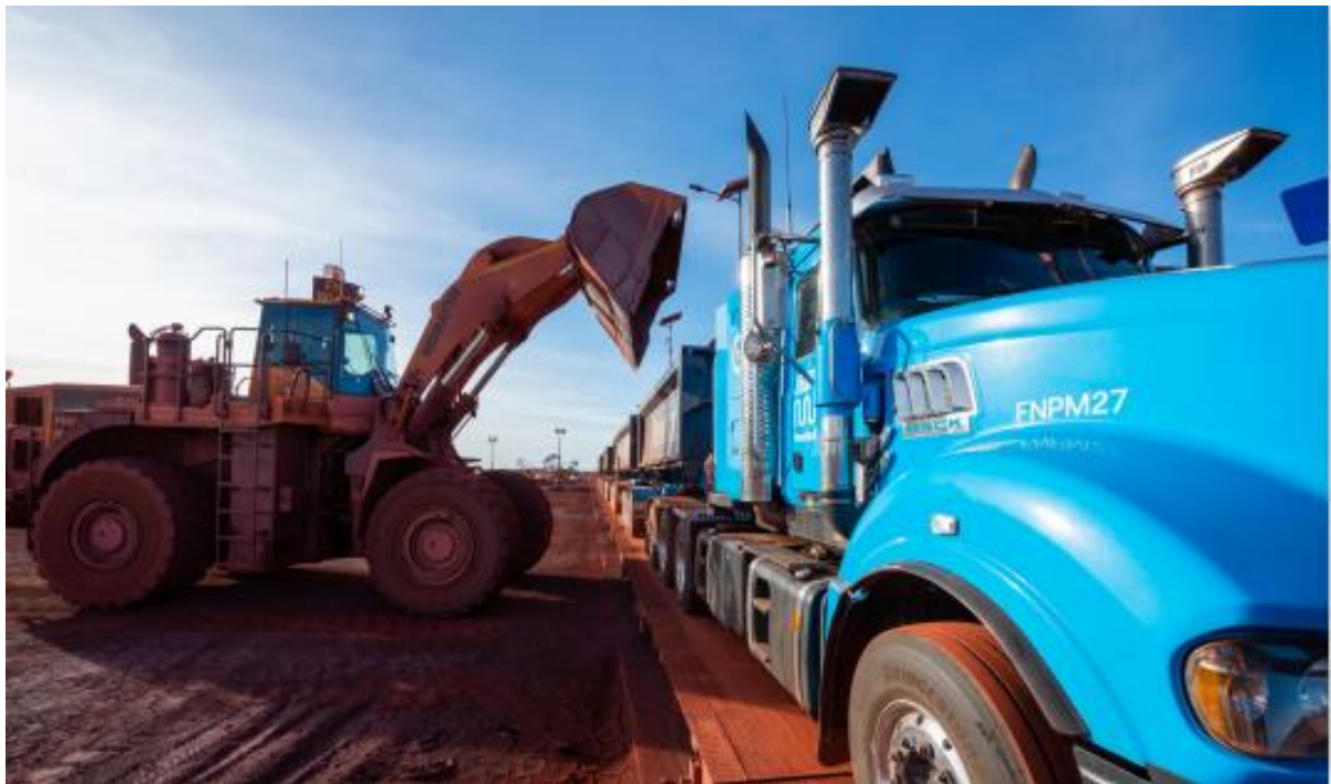
Fenix-Newhaul 200-tonne quad road train
