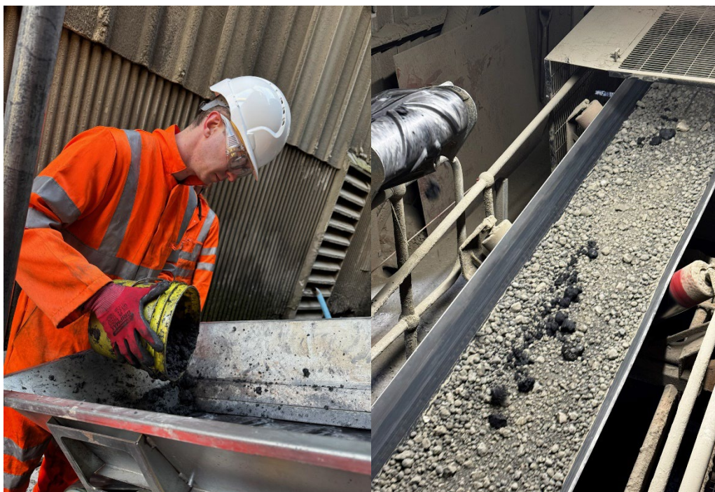
Figure 1. Graphene was added via conveyor belt to the cement production line.
