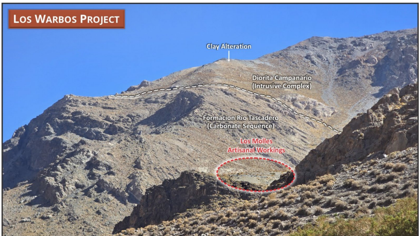
Photo 1. Looking west across Los Molles artisanal mining area, showing the contact between the marine carbonate sequence and a dioritic intrusive complex. Magnetic anomalies Warbos VIII to Warbos X are located behind the mountain and clay alteration. 4
