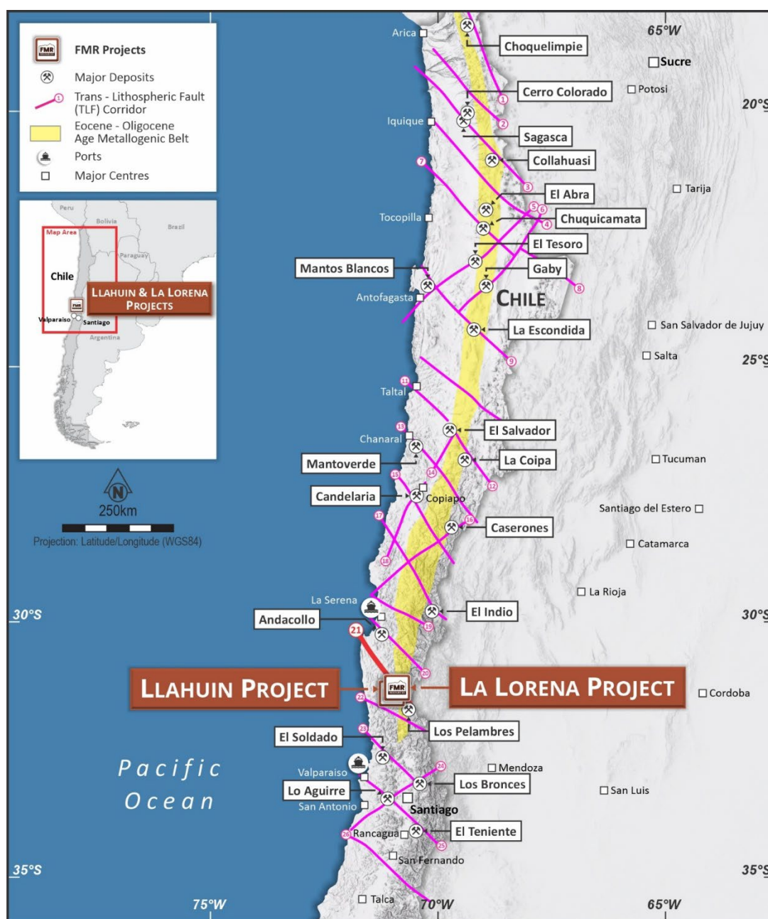
Figure 5. Map showing the La Lorena Project in the context of regional Eocene–Oligocene metallogenic age belt, major deposits, and regional structural architecture related to major deposits (after Rivera y Yañez, 2019).
