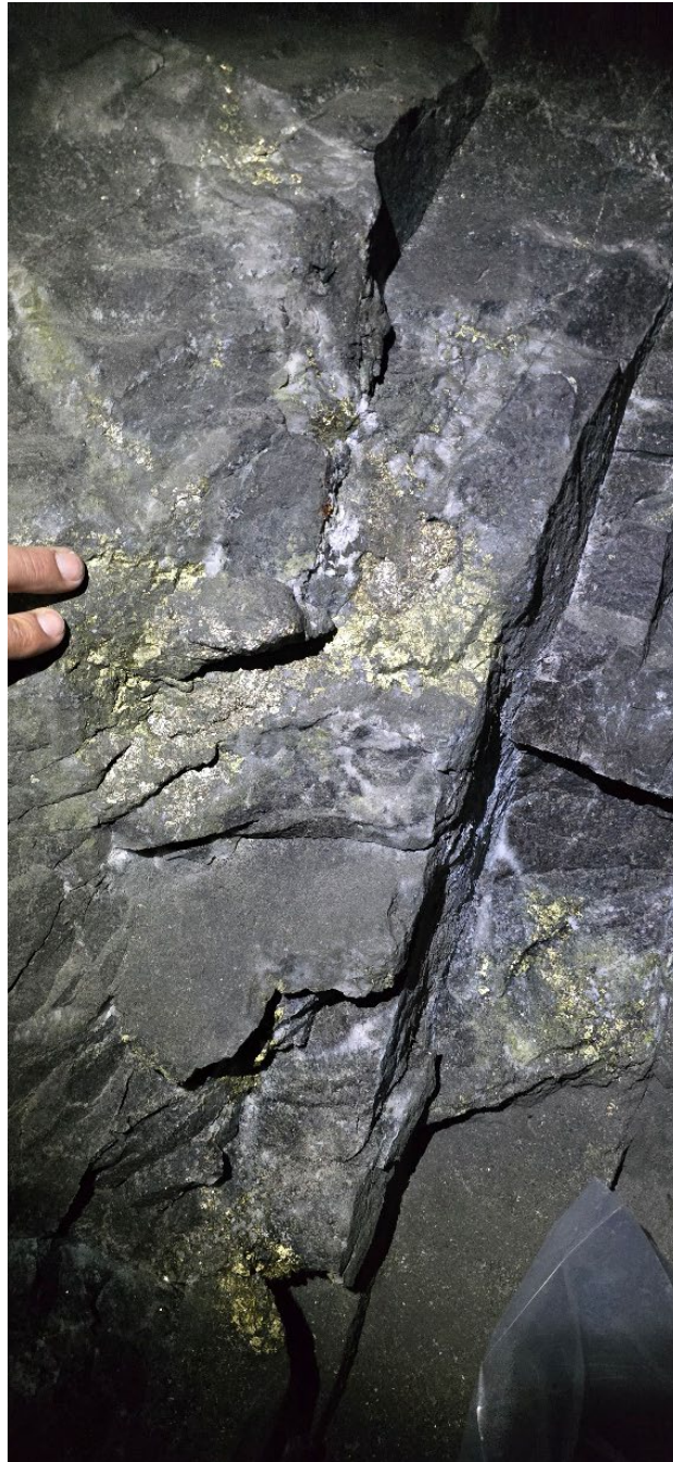
Photo 4. Underground mineralisation from the Los Morados Prospect, showing copper sulphide hosted in structurally controlled quartz-sulphide veining* (see Table 2).
