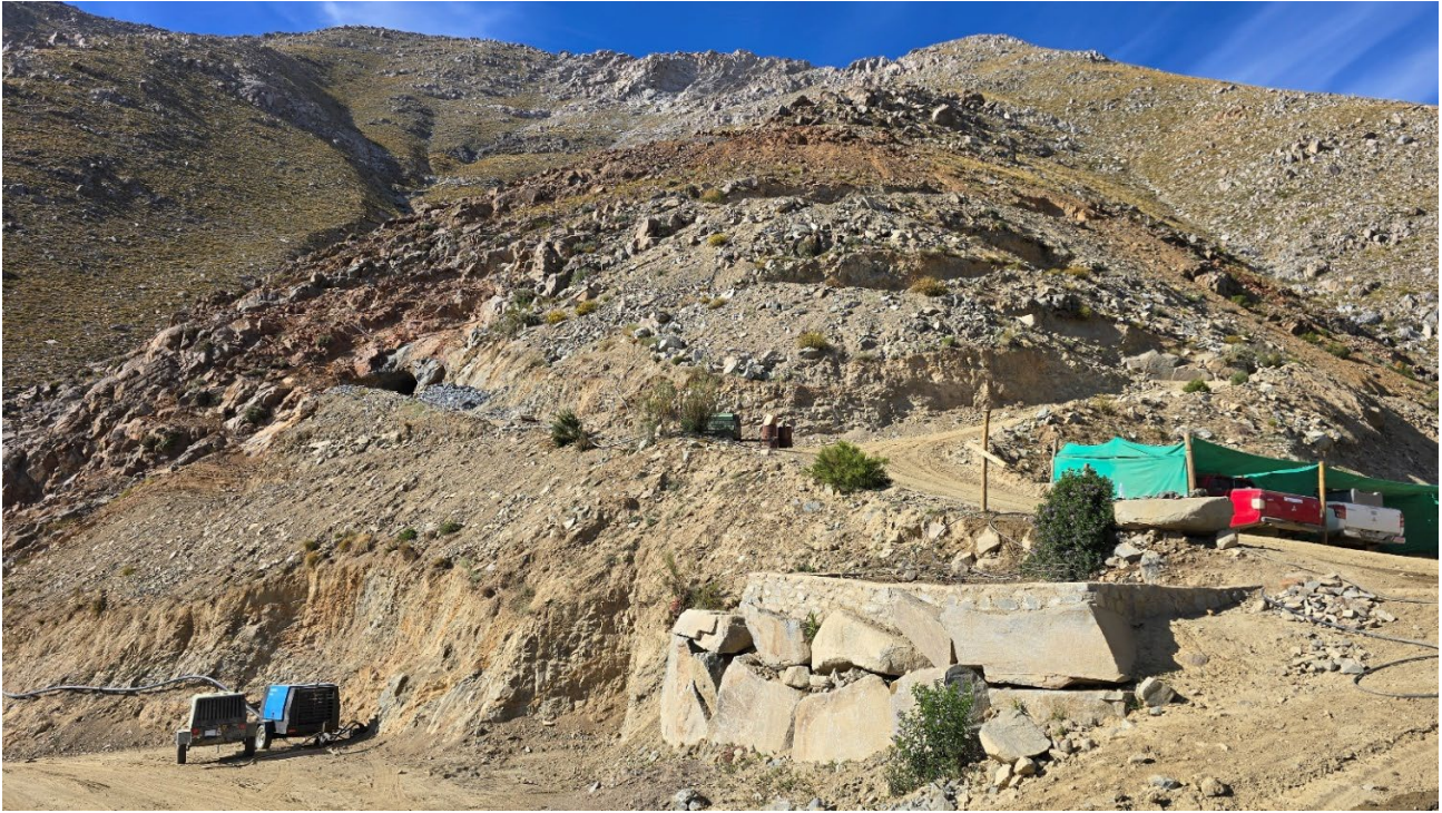
Photo 10. Mining operations at the Los Morados prospect, looking south towards the La Martuca Prospect, showing one of the 5-level adit collars centre left below the red oxide exposure of the mineralisation centre rear left to right.
