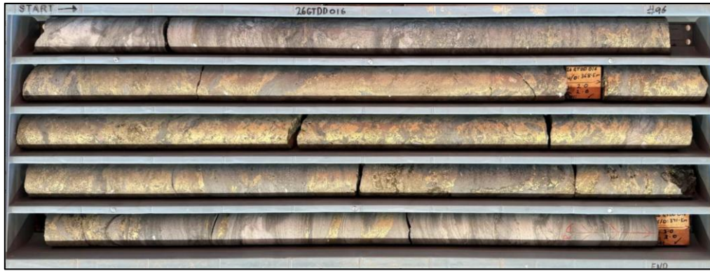
Photo 1: Core tray showing mineralised diamond core from drill hole 26GTDD016
