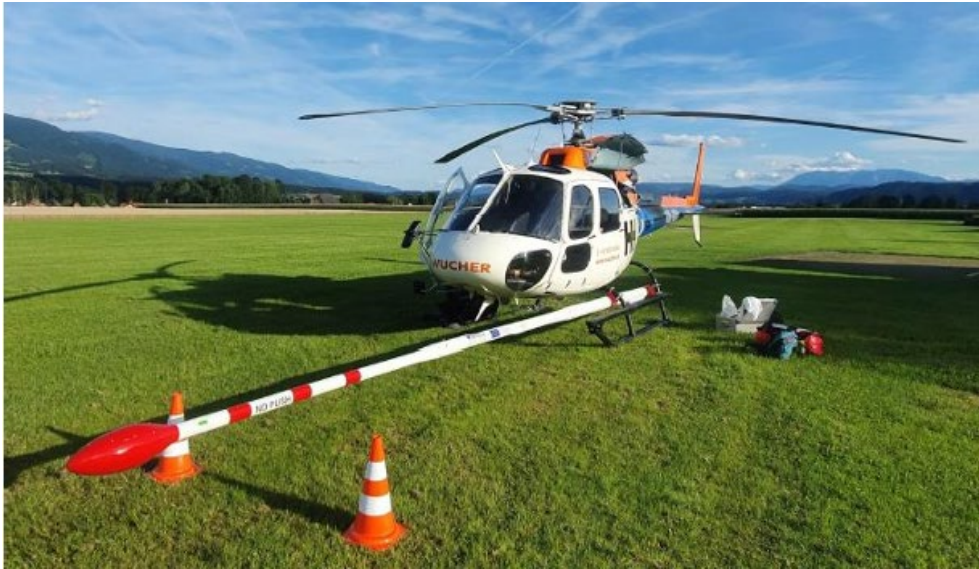
Nose boom magnetic and radiometric configuration on helicopter
