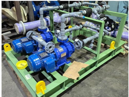
Filtrate Return Pumps Skid
