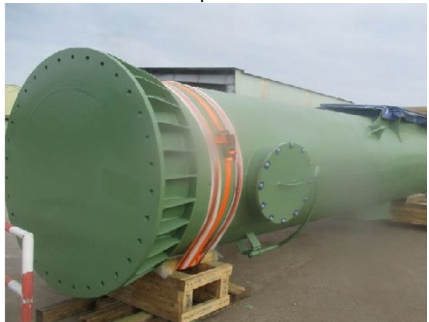
Main Venturi Scrubber
