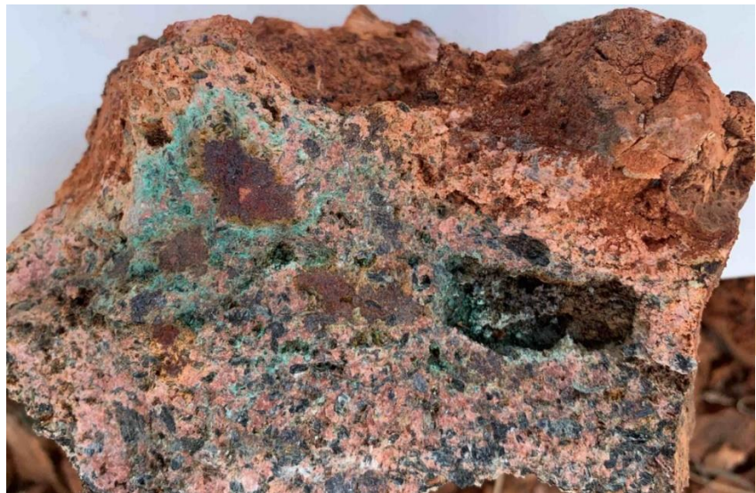
Copper mineralisation at Shadow within strongly altered Mt Philp Breccia (MJB490)
