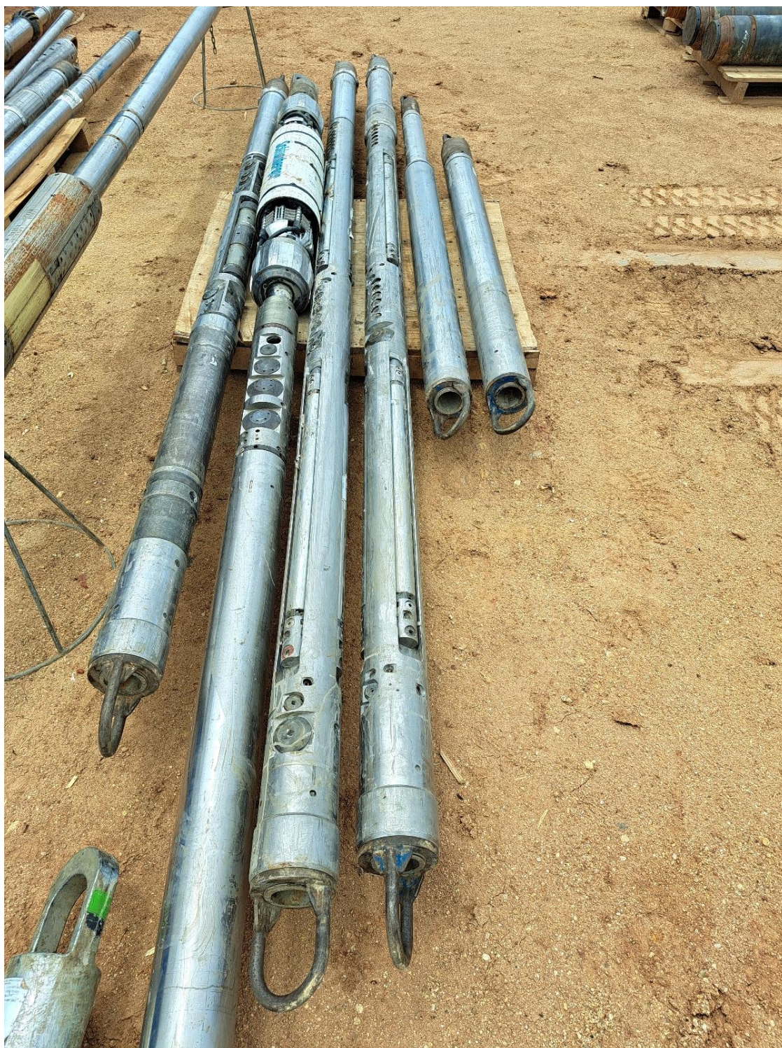
Figure 2 - Wireline formation sample tool and sample chambers at surface
