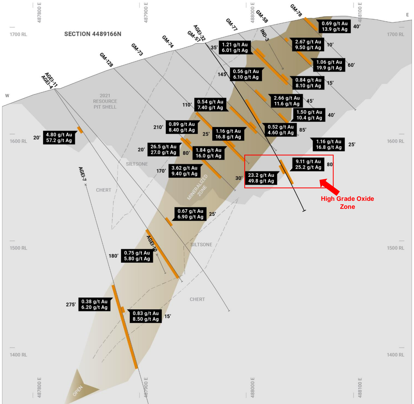
Figure 1 – Near-surface cross-section with high-grade oxide zone (within red box currently outside the existing NI 43-101 Mineral Resource).
