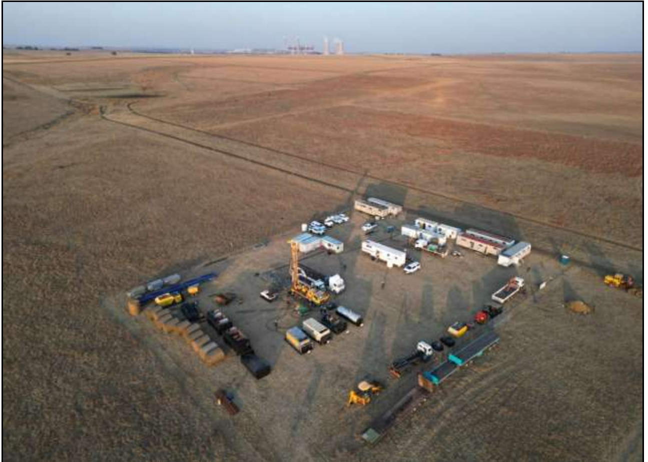
Figure 2 – Production drilling rig on site for spudding well 271-23PT with Majuba power station in the background.
