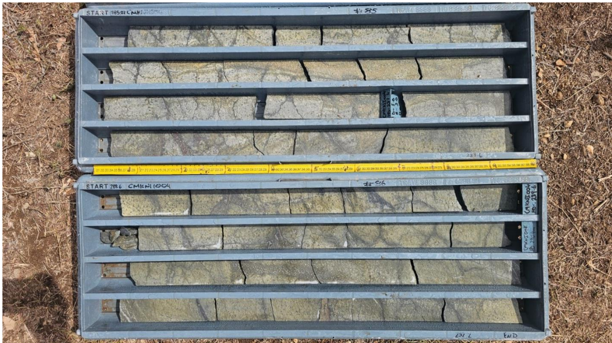
Figure 3: Diamond drill core (HQ) from hole CMKNI004 from 285.02m to 292.2m, showing stockwork style arsenopyrite-pyrite-proustite stringer veins within sericite-altered rhyolite porphyry.
