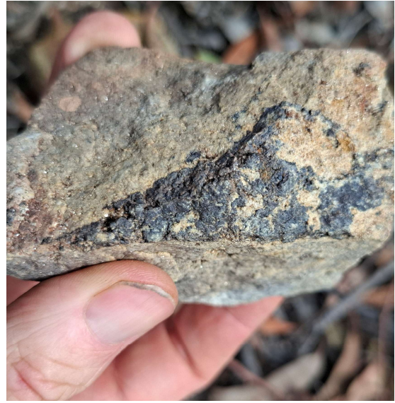
Photos 1 & 2. One of the historical mine shafts at the Dead Finish Mine at the Stannary Hills Tin-Tungsten Project and Sample KB072 showing cassiterite (tin) mineralisation from the Lass O’Gowrie Prospect that recently assayed 3.2% Sn.
