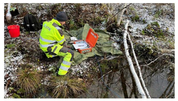
Figure 2: Installation of magnetotelluric measuring equipment
