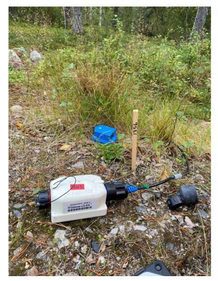
Figure 3: A geophone for seismic measurement of a dense network installed in the terrain.
