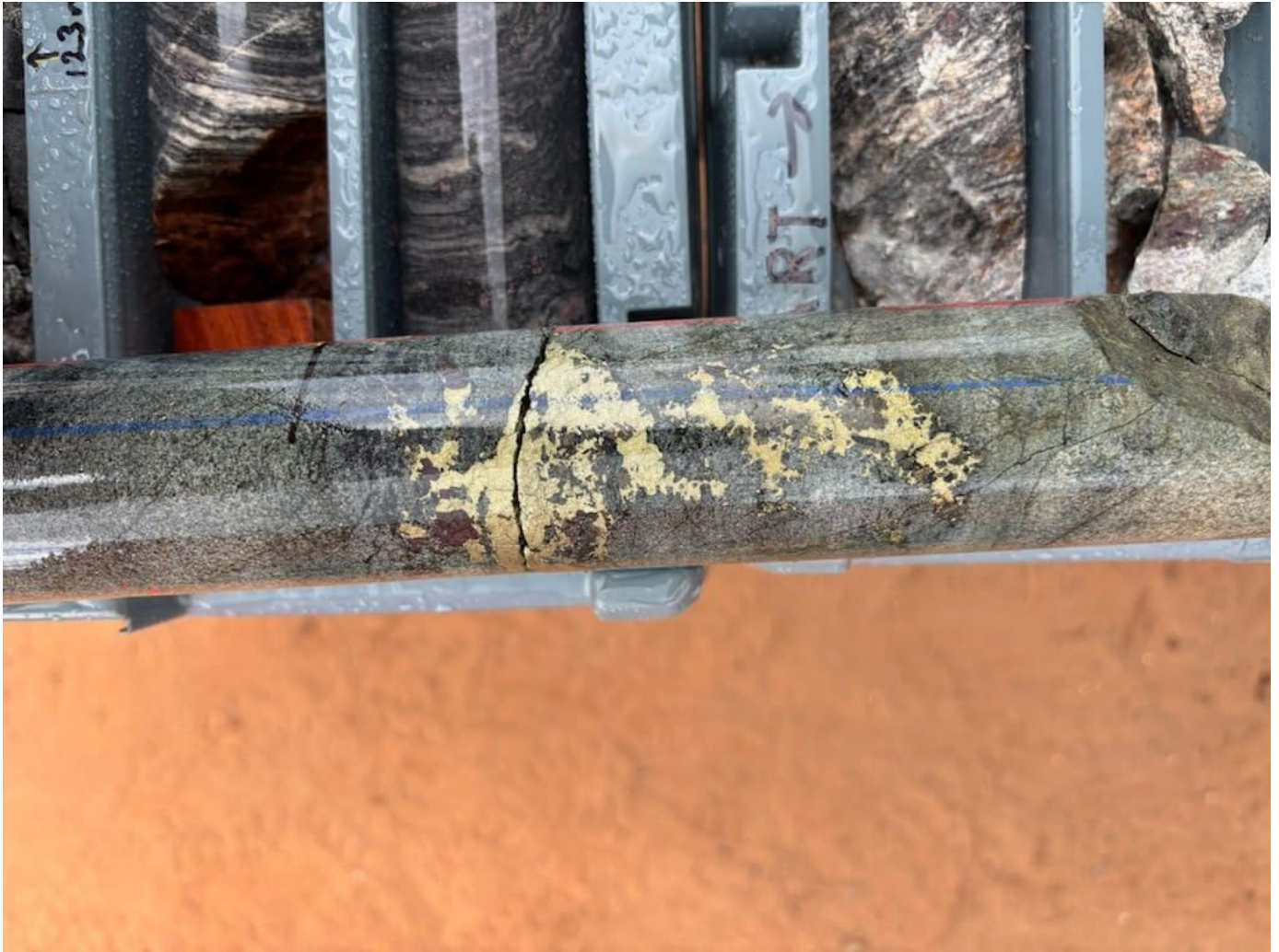
Figure 2. Diamond drill core from 158m downhole depth in OGDD002 assaying 1m at 3.1% Cu and 0.9% Zn.
