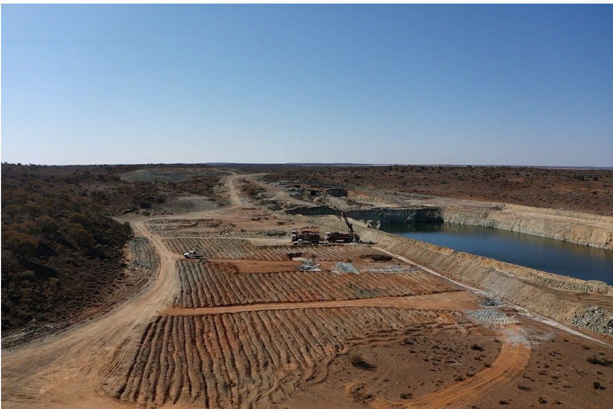
Figure 10: Aerial view of Devon Pit Gold Mine looking north towards Red October and Sunrise Dam Gold Mines showing the pit lake that requires dewatering
