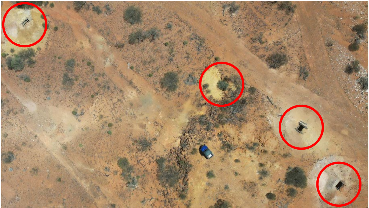
Figure 6: Drone image of Bunarra (Shaft 1) showing four shaft collars. Historical diamond drilling intersected significant gold in the north-northeast splay orientation, including 8m @ 21.99g/t Au (BN003).
