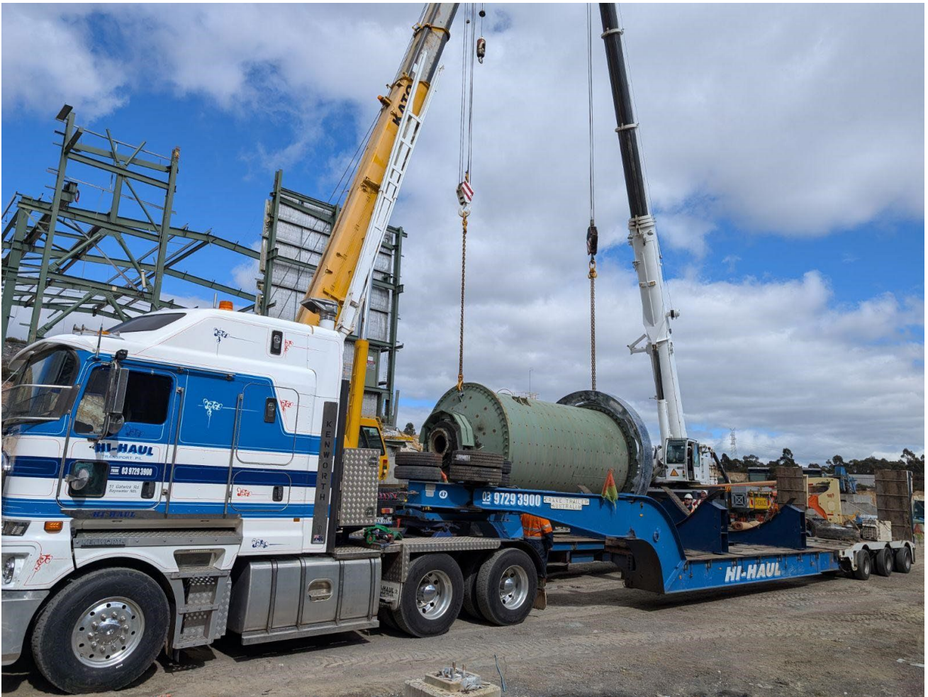
Figure 1: The 750kW ball mill being loaded for transport to the Murchison.
