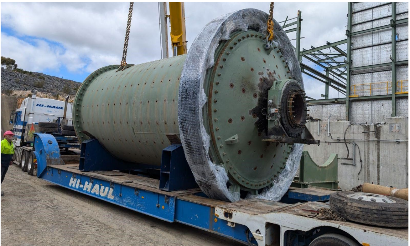
Figure 2: The 750kW ball mill being loaded for transport to the Murchison.
