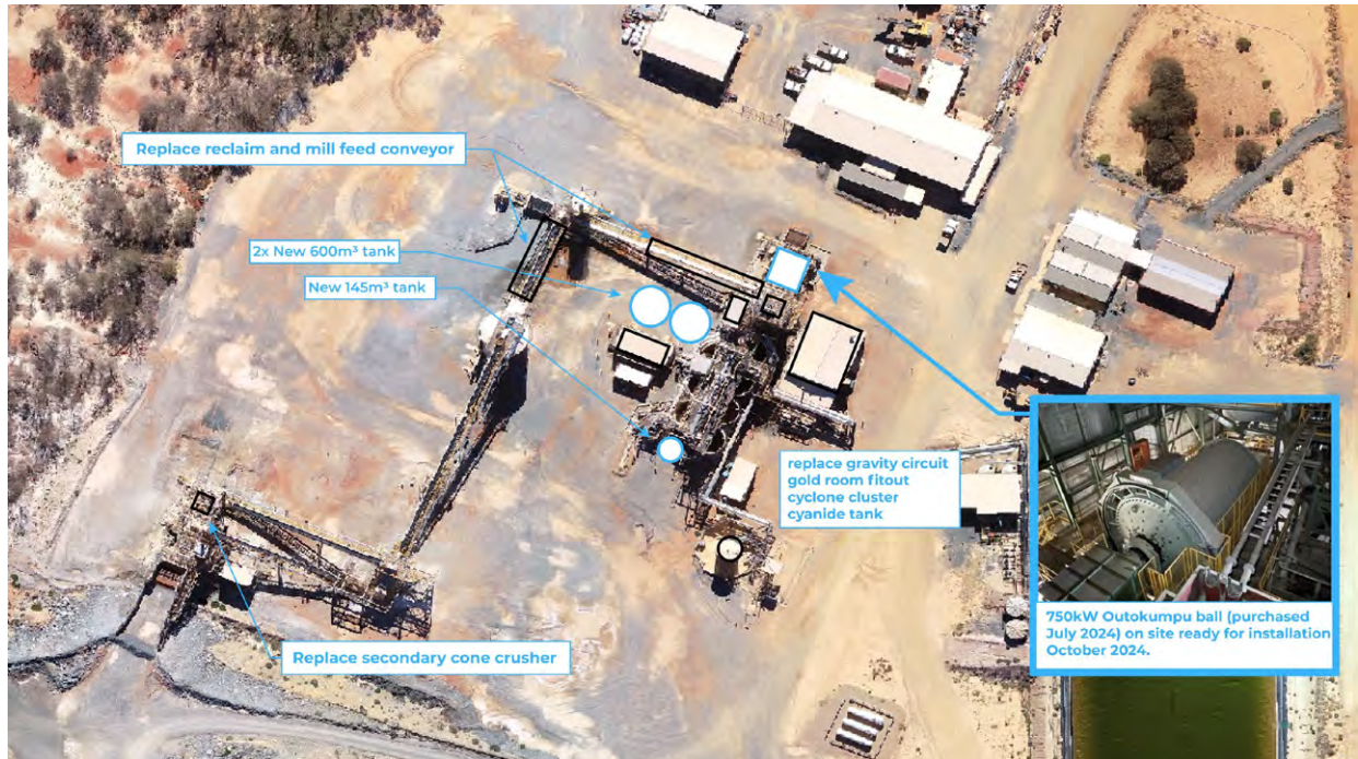
Figure 3: Process plant layout including upgrades.
