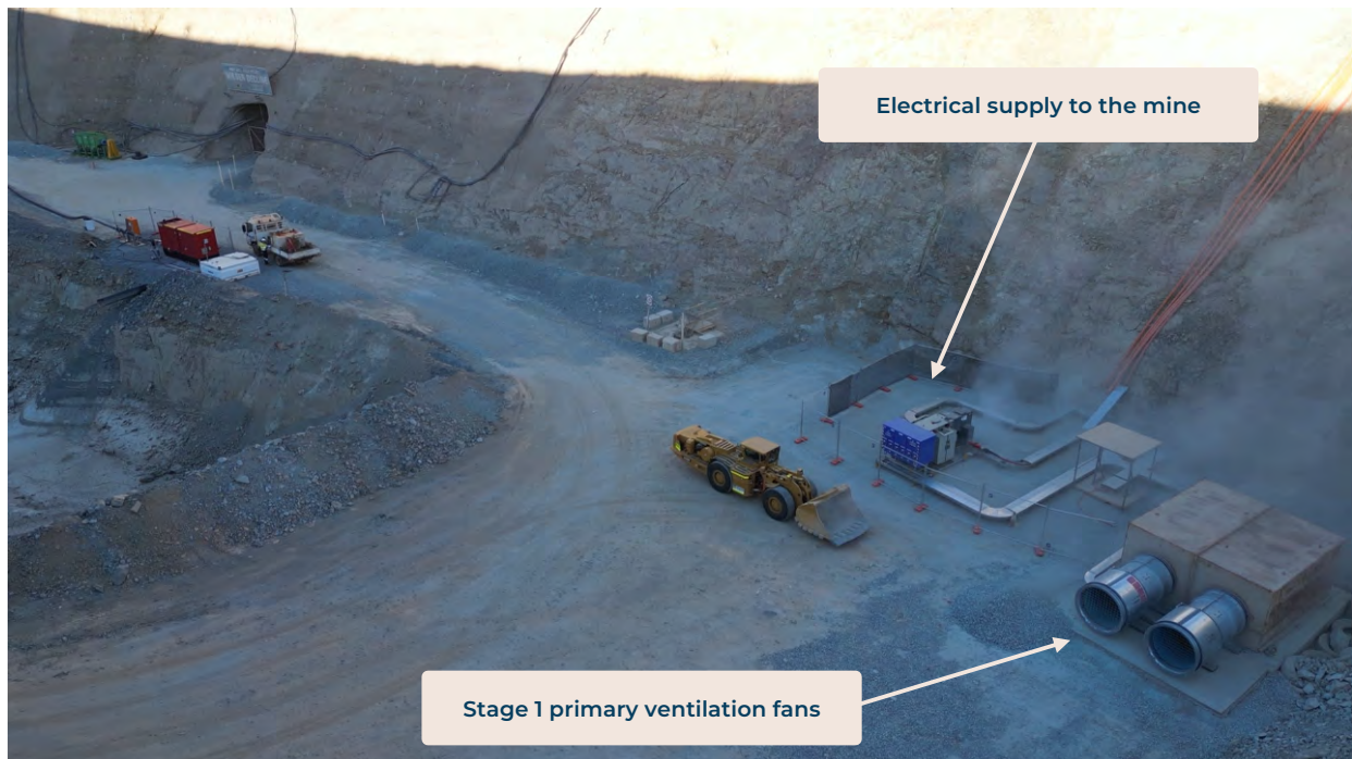
Figure 8: Ventilation, power and mine services established to the Andy Well underground.
