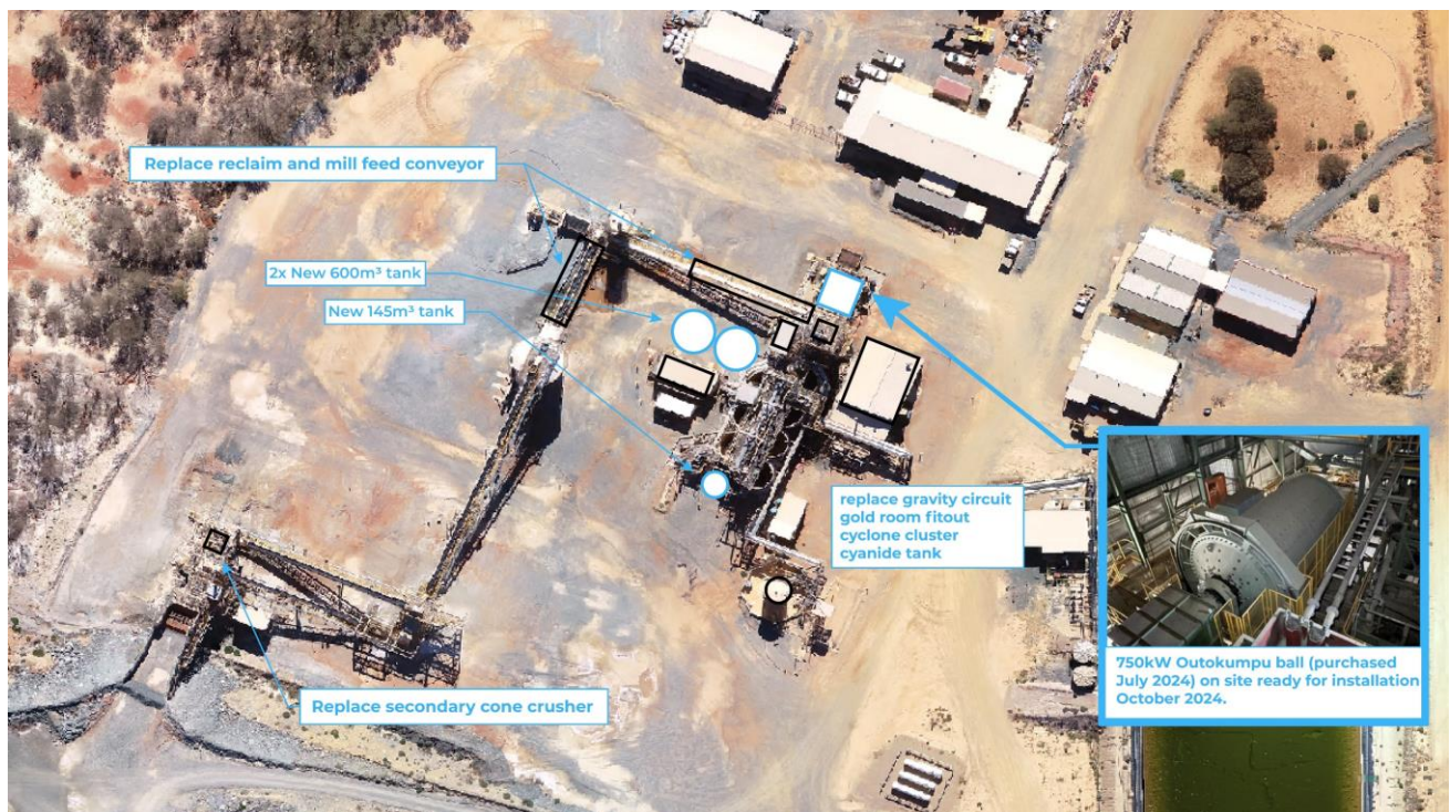
Figure 38 – Andy Well CIL process plant layout.
