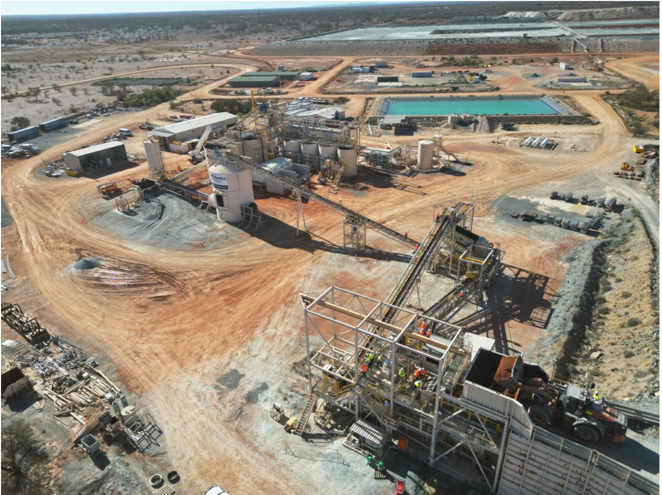
Figure 2: ROM loader feeding ore into the processing plant, 11 June 2025.
