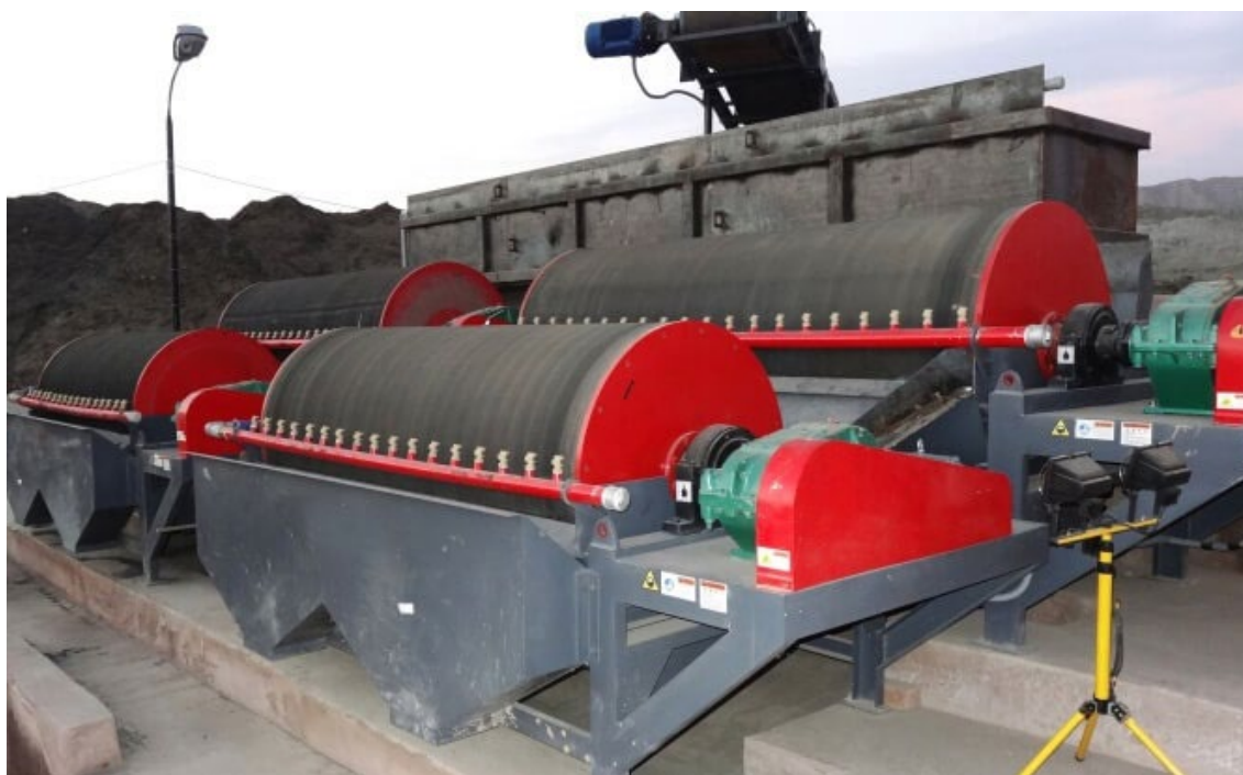
Figure 4 – Conventional magnetite beneficiation technologies will be used for ore processing including wet magnetic separation (stock image).
