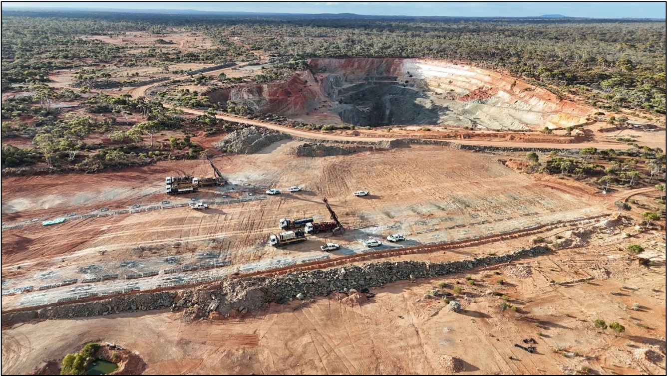
Figure 3: Grade control drilling (10m x 10m spacing), with the historical Phoenix pit in the background
