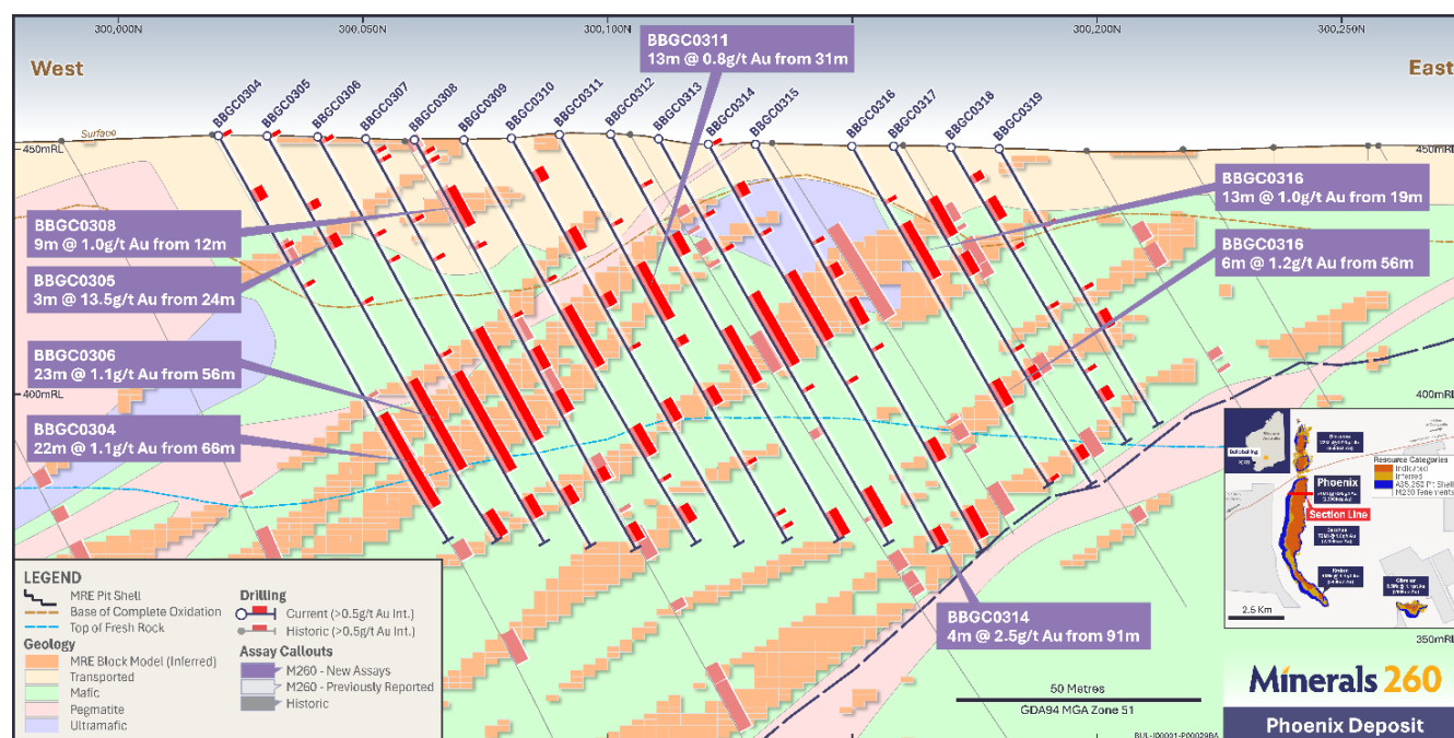
Figure 7: Section 6568350N showing mineralisation reported in grade-control drilling testing the Phoenix MRE pit shell compared with MRE Block Model (new results in purple boxes)
