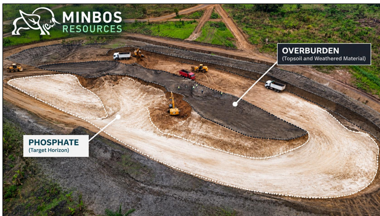
Figure 1: Aerial view of open-cut bench development and haul-road alignment at the Cacata Phosphate Deposit.
