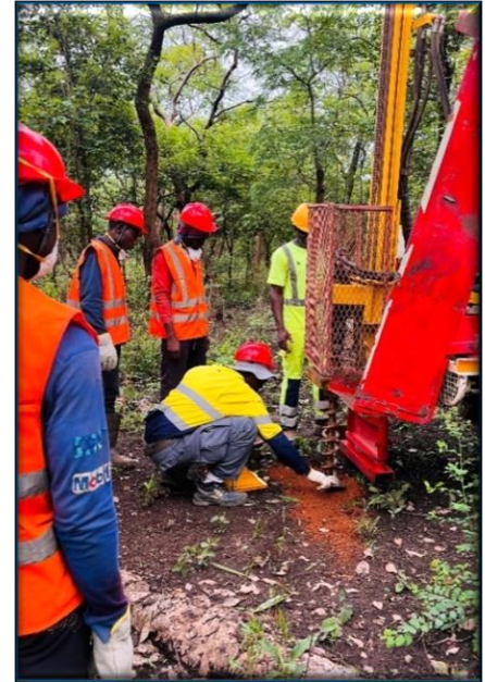
Figure 3 | Auger sample collection at Odienné Project, June 2024
