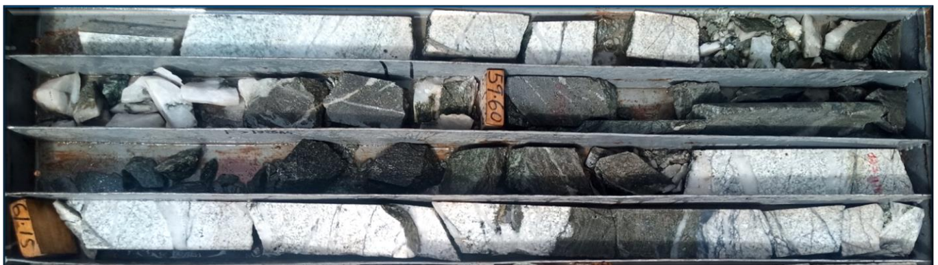
Figure 8 | Ferké diamond hole FNDC008, 58.18 to 62.1m Interval, where fire assays returned 1.5m @ 13.75g/t gold to 58.9m, 1.5m @ 6.57g/t gold to 60.4m, 1.5m @ 12.7g/t gold to 61.9m and 1.5m @ 0.36g/t gold to 63.4m drill depths
