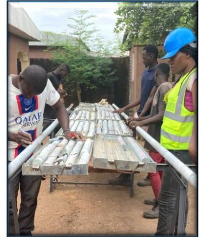
Figure 5 | Odienné Project diamond core processing - oriented core
