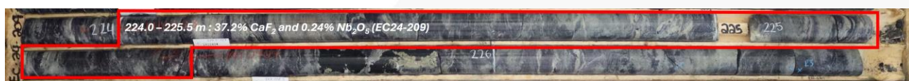
Figure 4. Example fluorspar (dark purple) mineralization in host dolomite carbonatite (light grey) at the Flux Fluorite Zone, Mallard Prospect (EC24-209; 2024 drilling campaign). The interval shown contains approximately 37% fluorspar (fluorite), with the remainder being predominantly dolomite.
