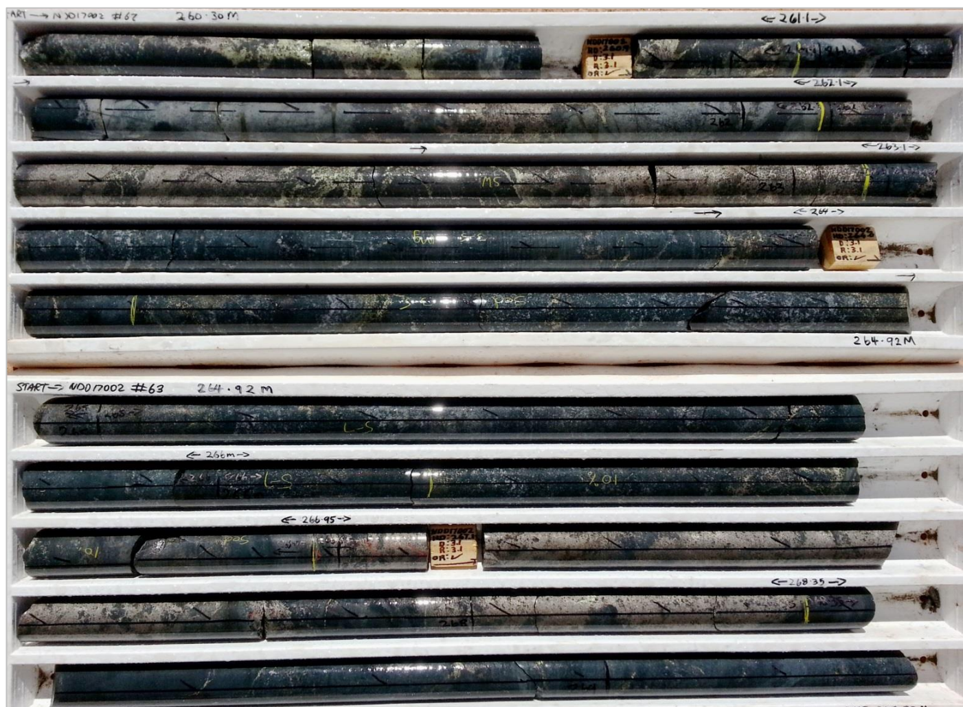
Figure 2: NDD17002 – 260.30 to 269.33 metres showing matrix, semi-massive and massive sulphide.
